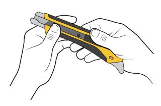
Push down on slider assembly and slide towards back end.
