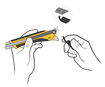
Slide new blade into channel. Align blade by placing the hole in the blade over the raised mounting point on slider assembly.
