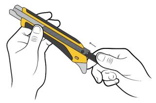
Push slider assembly and blade forward in handle to lock into place.
