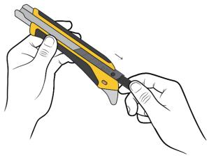
Push slider assembly past the base of handle to remove.
