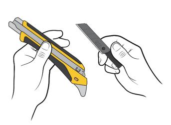
Remove slider assembly from blade.
