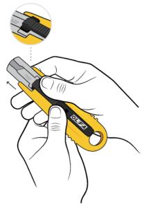
Push slider forward until black "wings" are centered in channel opening.
