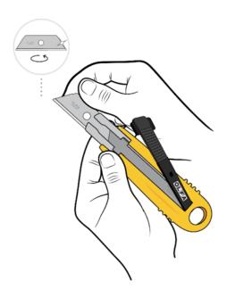
Carefully remove used blade. Flip endto-end for new edge or rotate 180° for left-handed use. Dispose of fully used blade properly in sharps container.
