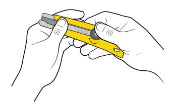
Turn ratchet-wheel dial counter-clockwise to loosen locking mechanism.
