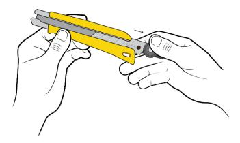
2 Slide ratchet-wheel assembly past base of handle to remove.
