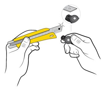
Insert new blade into channel. Align with assembly by placing the hole in the blade over the raised mounting point.
