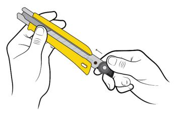
Slide ratchet-wheel assembly and blade forward.
