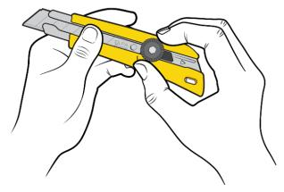
Turn ratchet-wheel dial clockwise to tighten the locking mechanism and return to work.
