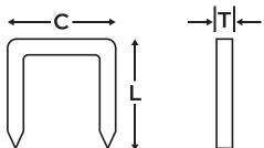
LENGTH: 10mm CROWN: 10.8mm THICKNESS: 1.25mm
