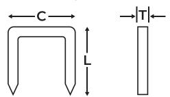
LENGTH: 6mm CROWN: 10.8mm THICKNESS: 1.25mm
