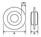
**BARCODE:** 8422514600514 **DIAMETER (d):** 19mm **DEPTH (D):** 6.2mm
