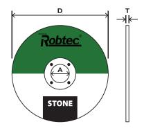
BARCODE: 9419678360117 DIAMETER (D): 115mm THICKNESS (T): 3.2mm ARBOR (A): 22.2mm **COLOUR:** Green **APPLICATION:** Stone/Masonry **ABRASIVE GRAIN:** Silicone Carbide GRIT SIZE: 30 HARDNESS GRADE: R STRUCTURE: 4 BONDING: BF (Synthetic Resin Bonded with Fibreglass Net Reinforcement) **SHAPE:** Flat **SPEED:** MAX. 13,290 RPM WORKING SPEED: 80 m/s WEIGHT: 60g
