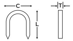
LENGTH: 11mm CROWN: 6.3mm THICKNESS: 1.2mm
